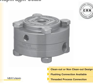
The Trerice **Threaded NPT Diaphragm Seal** is offered in both Clean-out and Non Clean-out designs, with female threaded connections of 1/4 NPT through 1 NPT. The Non Clean-out design can be furnished with diaphragm materials of Teflon (T), Viton (V), or Removable Metal (M), while the Clean-out design is available with all diaphragm choices, including Welded Metal (W).
